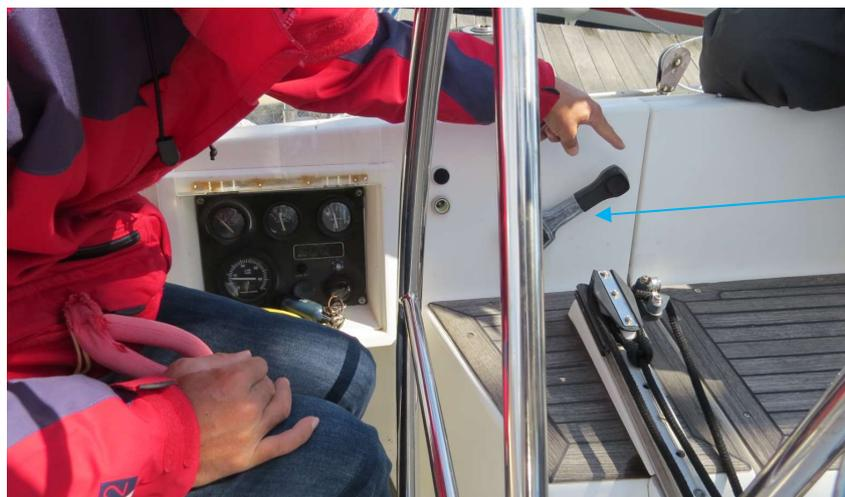
Engine Gear Lever
